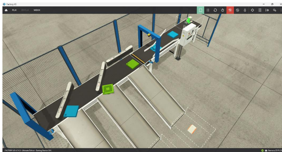
Fig. 10. Example simulation of product sorting in Factory I/O (own study)
