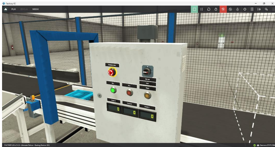
Fig. 8. View of the sorting line operator panel (own study)
