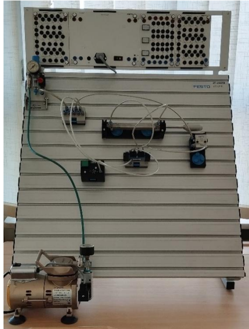
Fig. 5. Execution of the control system for the intermittent double-acting cylinder with the use of a 3/2 way roller lever valve and work cyclogram at the laboratory workstation Pneumatics TP 101
