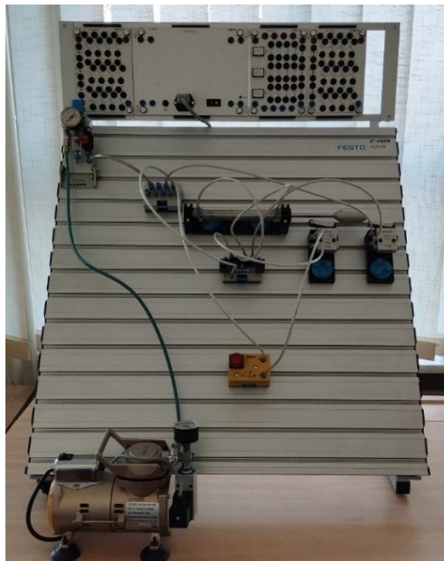
Fig. 7. The system executing the oscillating movement of the double-acting cylinder's piston rod performed at the Pneumatics TP 101 laboratory workstation
