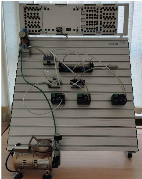
Fig. 9. The control system of double-acting cylinder with the use of AND at the Pneumatics TP 101 laboratory workstation
