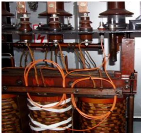
Fig. 11. Location of optical sensors (covered by white tapes)
