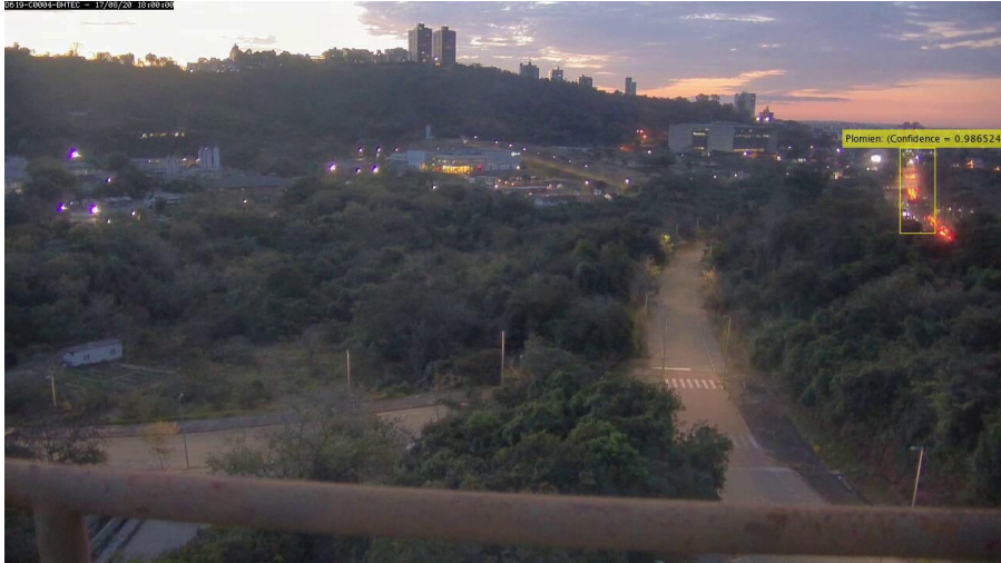
Fig 4. Example of False Positive caused by car lights.
