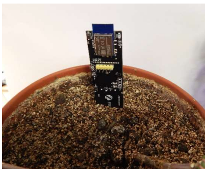
Fig.11 Zigbee Soil moisture sensor (author's photo)
