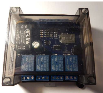
Fig.14 Zigbee relay module (author's photo)
