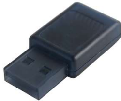
Fig.6 Z-wave network receiver-transmitter (author's photo)
